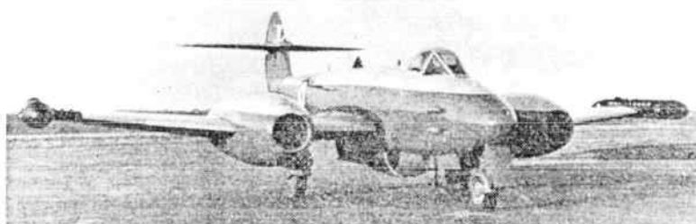
2) Wingtip camera pods and various command aerals were carried by RA421, the prototype U.15 target drone which was converted from a Meteor F.4.
